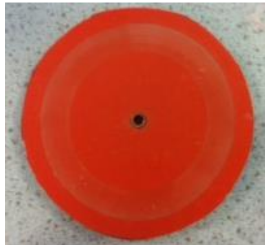
After Taber abrasion testing - Jogging Track (conditioned at 60°C, 30% Relative Humidity)
