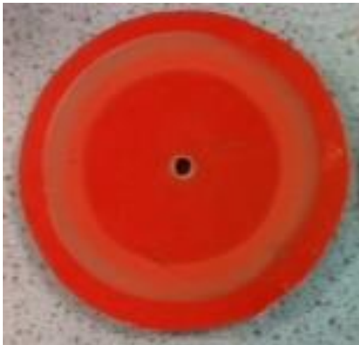
After Taber abrasion testing - jogging track (conditioned at 23°C, 50% Relative Humidity)
